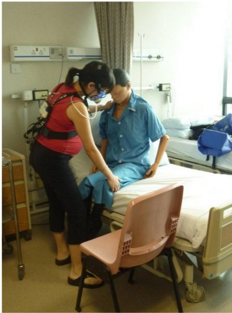
Fig. 1 Determination of average work intensity of Health care workers: In phase I pregnant subjects performed simulated patient care activities while breathing through a tight fitting mask with a pneumotachometer. Oxygen content was sampled at every breath and measured with a portable telemetric metabolic cart
